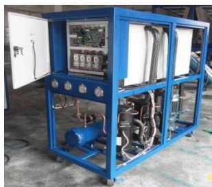
Gambar 4. Alat pengujian water chiller
