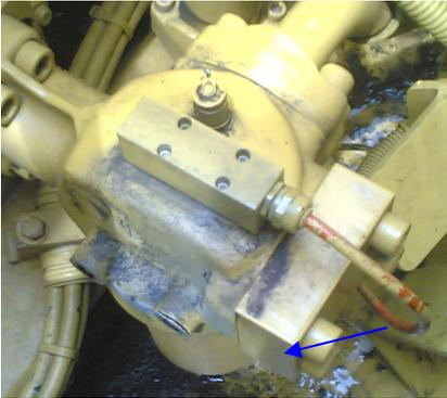
Gambar 3. High Pressure Filter.
