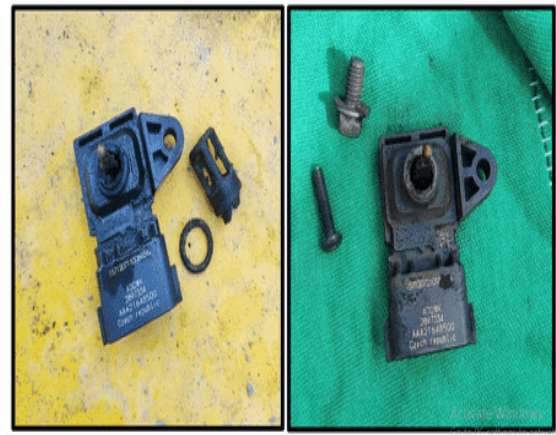
Gambar 6. Kondisi boost pressure sensor
