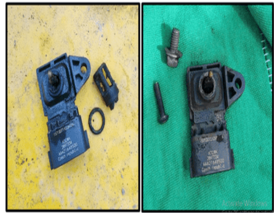
Gambar 6. Kondisi boost pressure sensor
