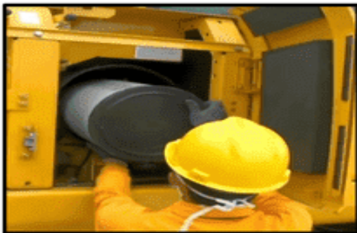
Gambar 8. Pengecekan air cleaner
