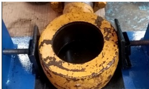
Gambar 16. Pemasangan special tool ke housing cylinder
