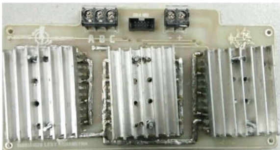
Gambar 9. Hardware rangkaian inveter tiga fasa
