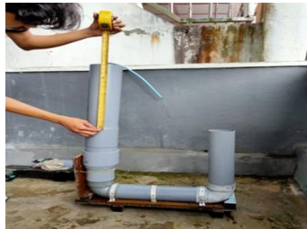
Gambar 5. Pengujian permeabilitas pervious concrete
