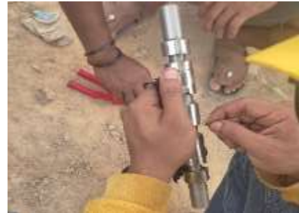
Gambar 8. Pembersihan spool counterbalance valve
