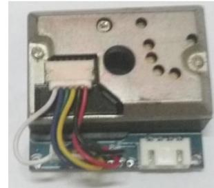
Gambar 6 Sensor Sharp GP2Y1010AU0F
