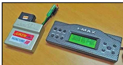
Gambar 4. ECU Programmable BRT Juken 3 Beat FI
