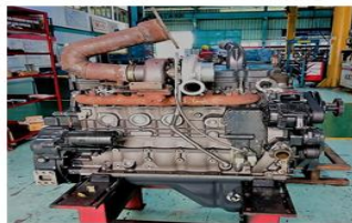
Gambar 1. Engine Komatsu SAA6D107E-1
